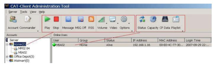
The command group is highlighted by the left rectangle and the current active group will be highlighted by the cursor. Pressing any button on the command group will result in a command being sent to ALL client devices under the active group. In this example, if we press "Stop", MP02 84 and MIA02 will both stop their video stream.
